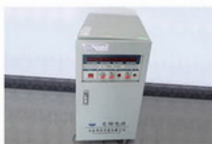
Switching Power (To Adjust Voltage and Frequency when conducting aging test)
